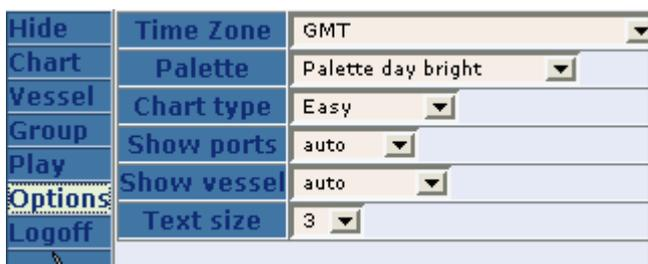
The point is used to select the mode of the optimum layout for the given working place. Here, it is possible to select the time zone, the pallet, the type of reflected chart - Synthetic or Navigation, the mode of layout of the ports (for the Synthetic chart), of the vessels and the size of the police for the inscriptions on the chart.
