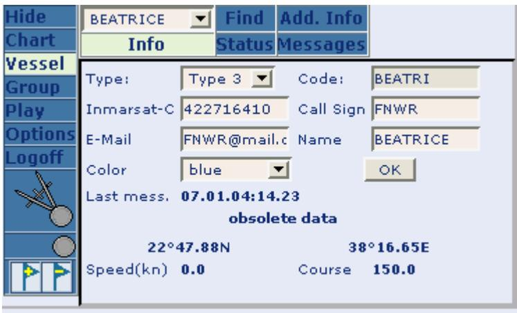
This point serves for mapping and correction of the information about the selected vessel (when the user has the appropriated privileges). The vessel is selected with the given list or by the mouse clicking on the image of the vessel on the chart.
