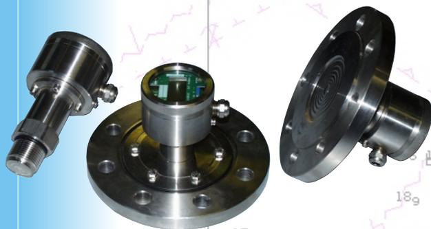
Pressure transmitters series 27, 86 and 93 utilize the piezo-resistive pressure sensor. It is a fully active Wheatstone Bridge of resistors diffused in a crystal silicone chip.
